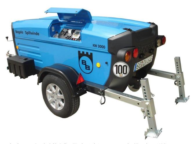
The approved and compact Bagela Cable Pulling Winches in their new cover, made of Terpolymer (ABS).
