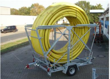
There is no bending tension on the pipe coil. The roll resistance is less than of conventional solutions. No more inner rollers are necessary and the inner end of the pipe can be pulled into the coil. The BRVT 16 is able to load and uncoil wider pipe coils.
