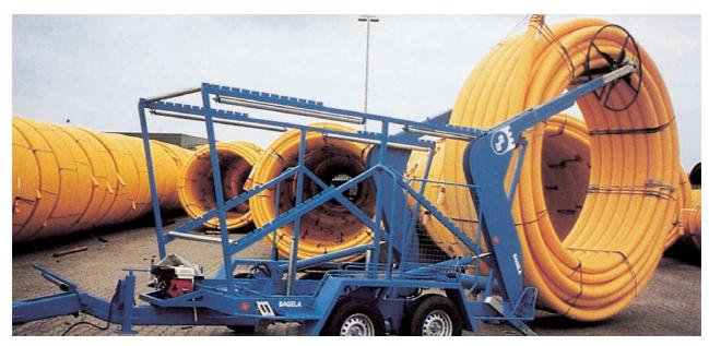
The BRT 20 is able to pick up, load and uncoil pipe coils without any help. Even laying coils can be picked up without any auxiliary equipment. Tube coils of varying diameters may be picked up with the aid of the vertical hydraulic jacks and put down on the bearing rollers. Then three guiding rollers are inserted on the inside of the coil, and the coil is ready for unreeling.
