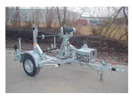
Cable drum trailer type BKT 10 with a hydraulic power pack (4 kW) and a single arm cable drum drive for fibre optic cables.
