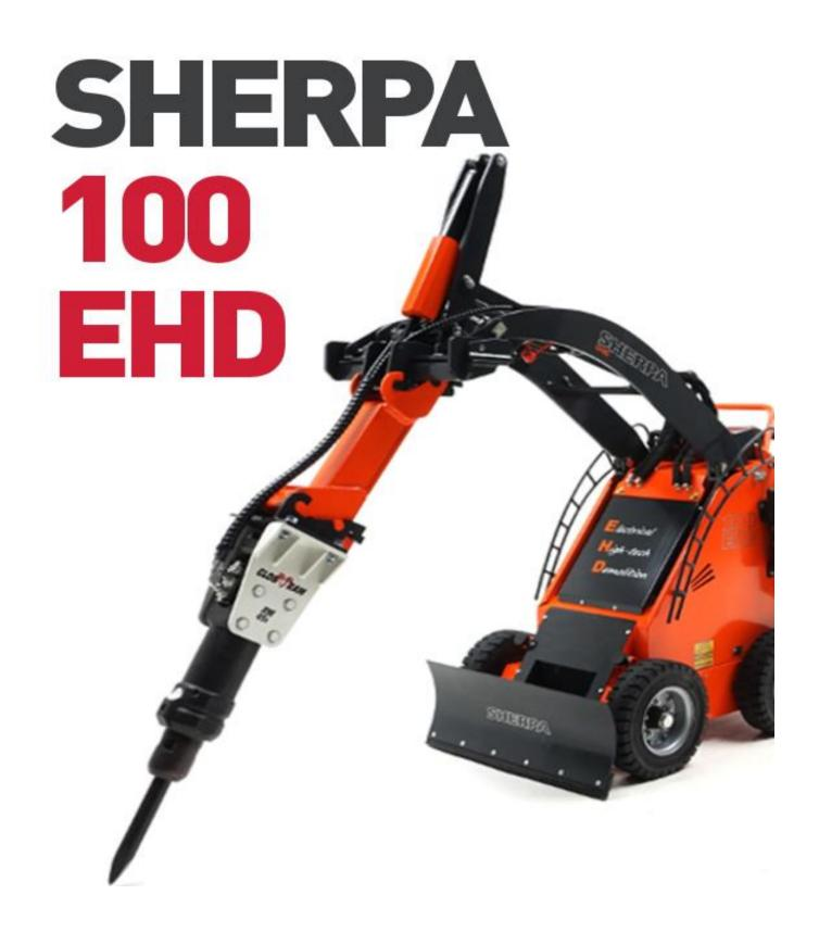
The SHERPA 100 EHD has all the features that make the SHERPA 100 ECO unique. In addition to the revolutionary electric motor, the SHERPA 100 EHD has radio control. This makes it possible to work in areas that are difficult to access and the desire to guarantee safety for professionals is met optimally.
