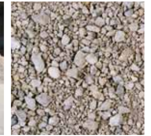
Recycled concrete aggregate
