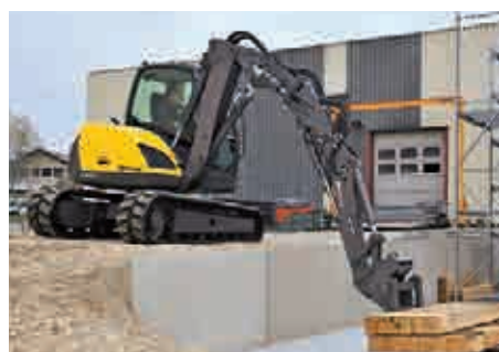
Handling with forks below the ground level, this is unique for an excavator.
