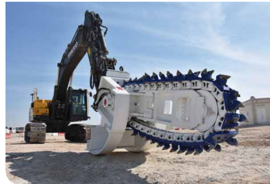
Qatar The new KEMROC trencher ETR 3 trenches 60 cm wide and up to 2 m deep in medium hard limestone. The trencher is mounted on an EC 380 Volvo Excavator.
