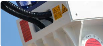
Housing with hydraulic hose protection.
