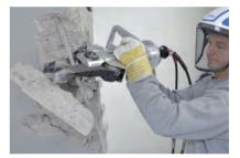
The HCS8 C is specially designed to expand and separate material, e.g. ripping radiators or door frames from walls or breaking up concrete pieces. The tool has a shear set for cutting-up various materials, like reinforcements up to 20 mm (0,8 inches) in diameter.
