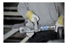
The HCS8 S, equipped with sickle shaped blades, is able to cut sheet metal, piping, high voltage cables, rebar (up to 16 mm/0,6 inches in diameter) and wooden frames. The sickle insures that the material can't slip out.
