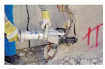
The HCS8 J is able to crush concrete walls up to 15 cm (5,9 inches) thick (depending on compression strength of the concrete). A big advantage for breaking, separating walls, facade or reclamation concrete panels.
